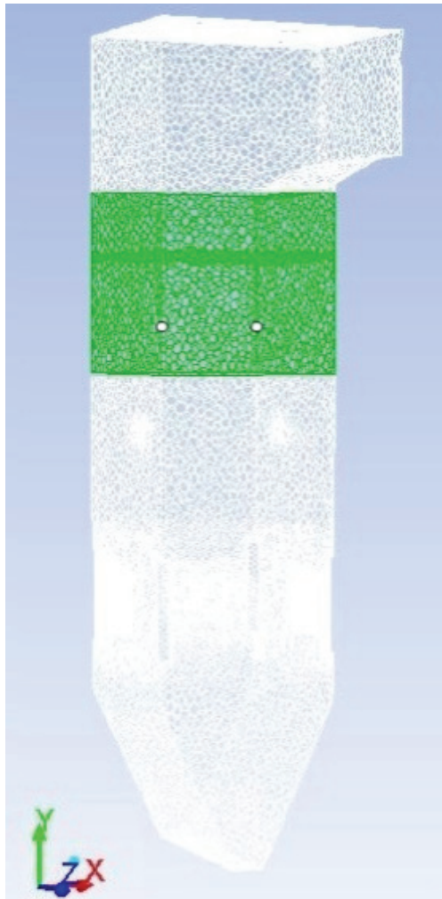
Figure 1: Computational geometry used to analyse the impact of injection parameters on reagent behaviour in the boiler volume (marked green)
