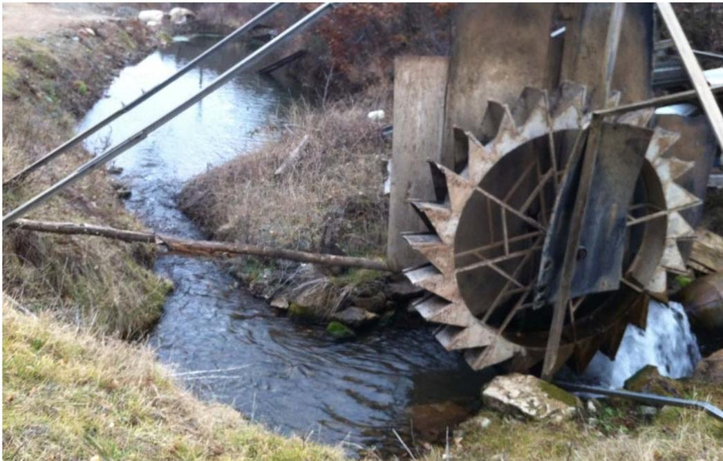
Figure 12: Old water wheel turbine for generating energy from water
