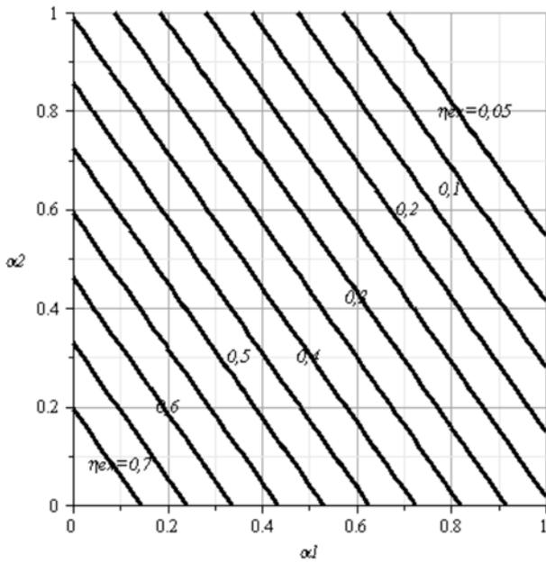
Figure 4: Exergetic efficiency  $\eta_{ex}$  as a function of  $\alpha_1$  and  $\alpha_2$
