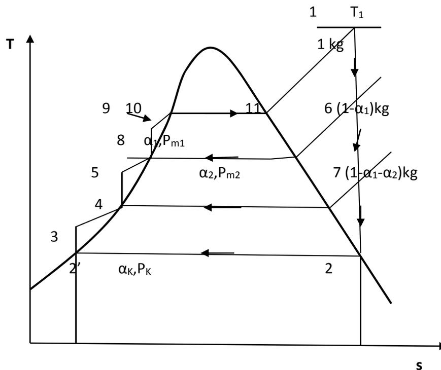
Figure 2: Regenerative heating process diagram (s, T)
