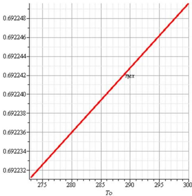
Figure 6: Exergy efficiency  $\eta_{ex}$  to EPP Kosovo B in function of temperature  $T_0$  (K) of the surrounding
