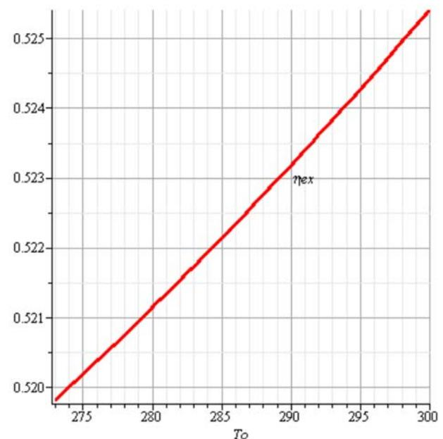
Figure 3: Exergy efficiency  $\eta_{ex}$  in function of temperature  $T_0$  (K) of the surrounding
