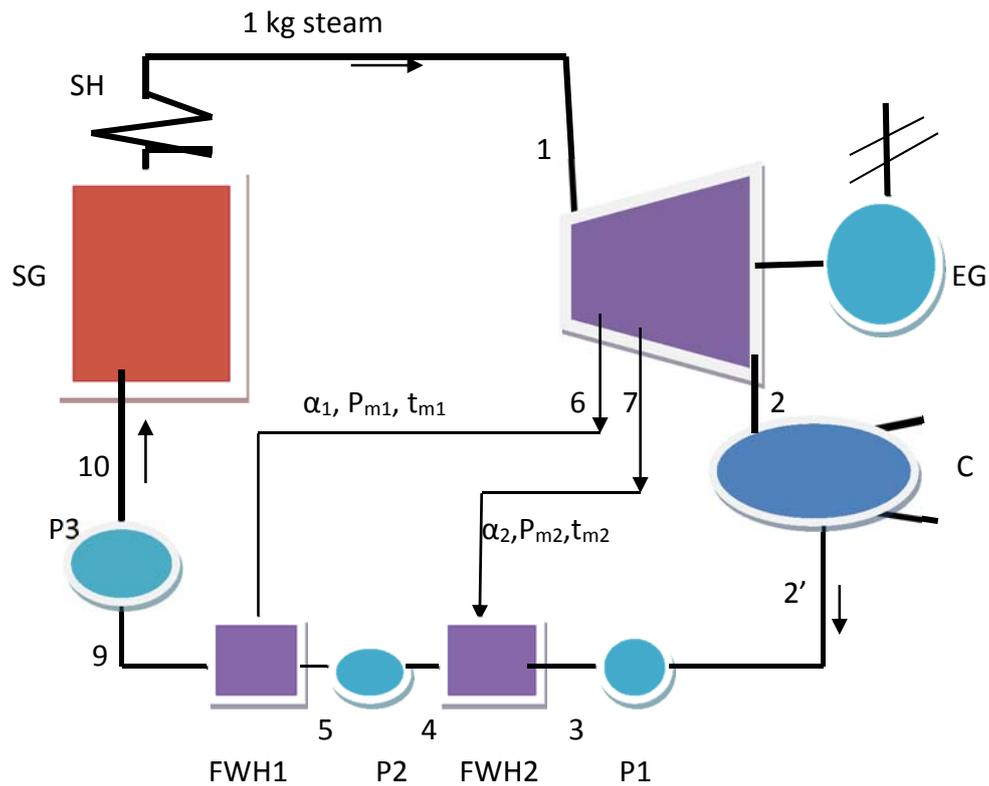
Figure 1: The Scheme of the regenerative heating of the feeding water:
