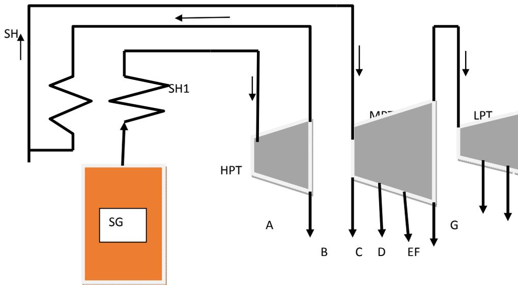
Figure 5: The scheme of the steam turbine for EPP Kosovo B (SG-steam generator, SH-super heater, SG- steam generator, HPT-high pressure turbine, MPT-medium pressure turbine, LPT- low pressure turbine)
