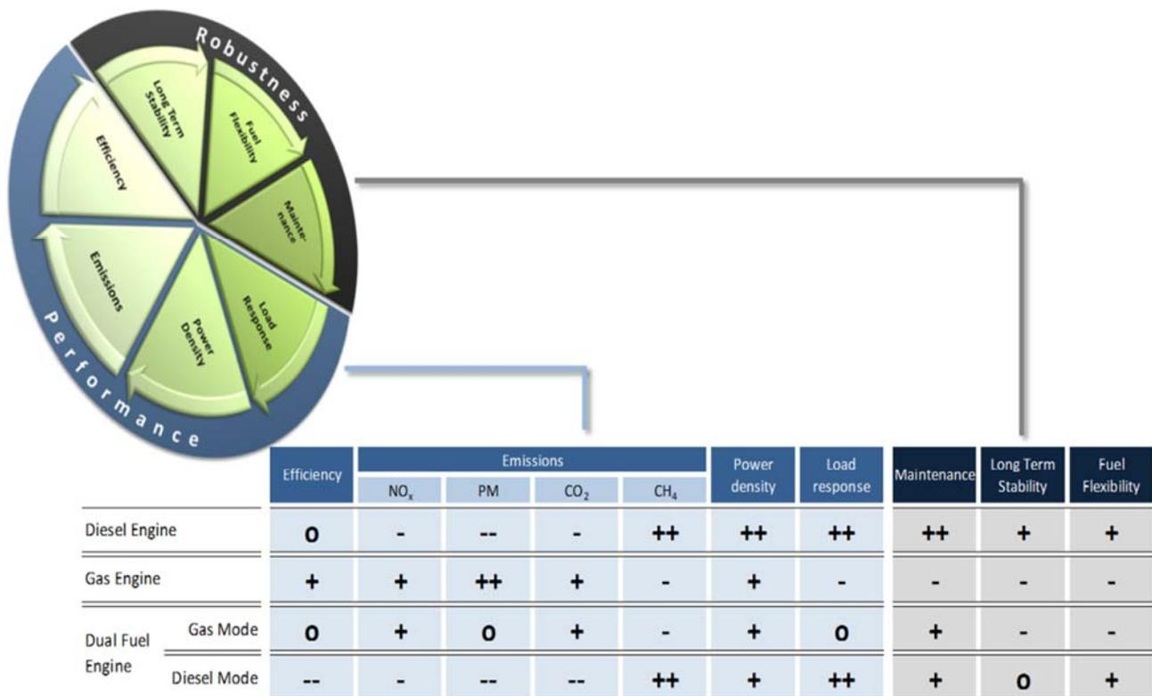
Figure 3. Evaluating engine technologies
