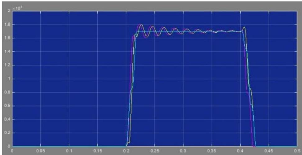
Figure 5. Fault current sec. for the 3-phase fault occurring at F4, case of non-parallel mode of transformer operation
