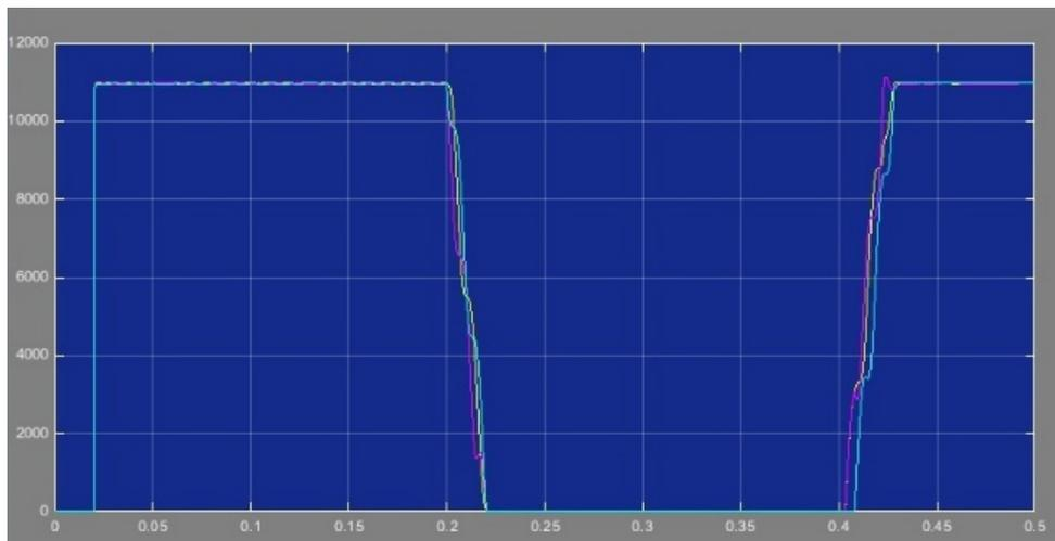
Figure 6. 3-phase fault rms voltage curve before, during and after the fault occurrence at F4 case of non-parallel mode of transformer operation
