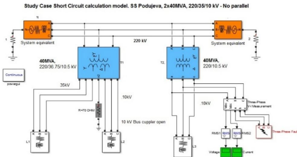
Figure 3. Schematic Matlab/Simulink block diagram for the fault analysis – case of non-parallel mode of operation – transformer inter-connecting power link switch open
