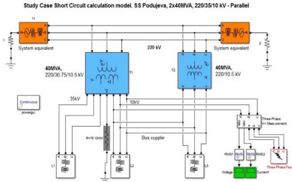
Figure 4. Schematic Matlab/Simulink block diagram for the fault analysis – case of parallel mode of operation – transformer inter-connecting power link switch closed
