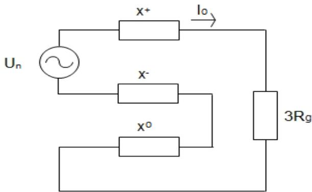
Figure 9. Network equivalent schemes for d, i, o sequences
