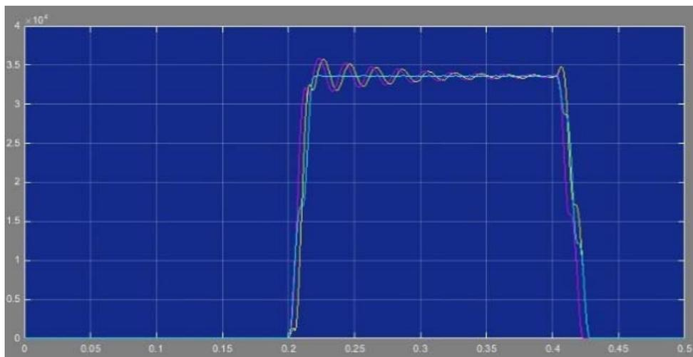
Figure 7. 3-Phase fault current at F2 for parallel mode of transformer operation
