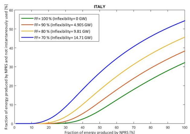
Figure 3. Energy yearly produced by NPRS that cannot be instantaneously consumed (Excess rate), expressed as a function of the fraction of energy produced by NPRS (NPRS penetration) for different  $FF$  values at National scale
