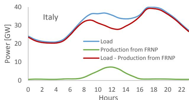
Figure 2. Typical load and NPRS generation profile for a sample day (January 3<sup>rd</sup>, 2013) [14]
