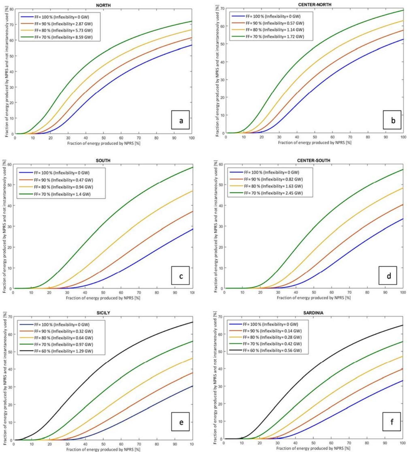
Figure 4. Energy yearly produced by NPRS that cannot be instantaneously consumed (Excess rate), expressed as a function of the fraction of energy produced by NPRS (NPRS penetration) for different *FF* values at area scale
