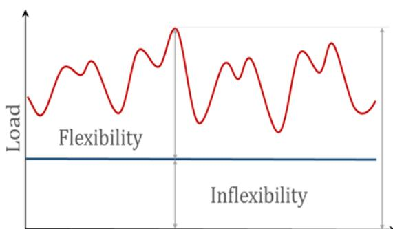
Figure 1. Definition of Flexibility / Inflexibility in an electric system
