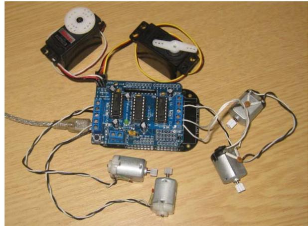
Figure 2. Arduino boards that can control up to 4 bi-directional DC motors with individual 8-bit speed selection, or 2 stepper motors (unipolar or bipolar)
