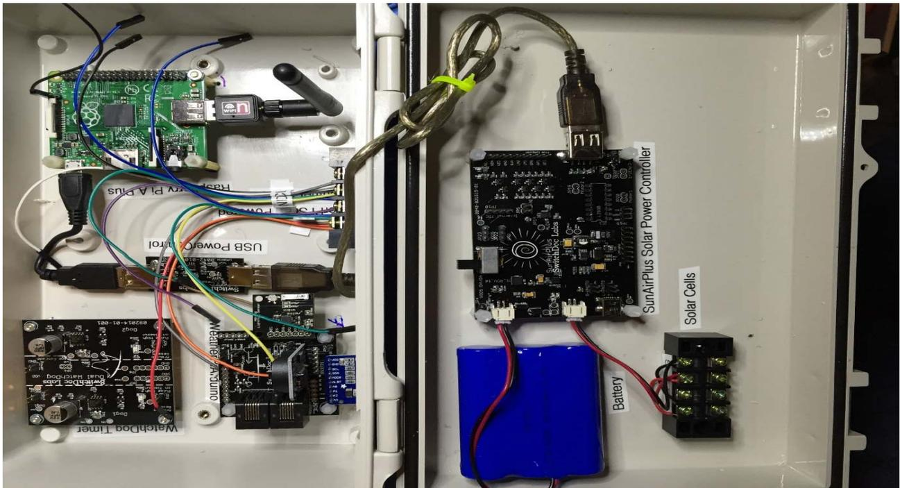
Figure 3. Solar tracking system built by WatchDoc Lab.
