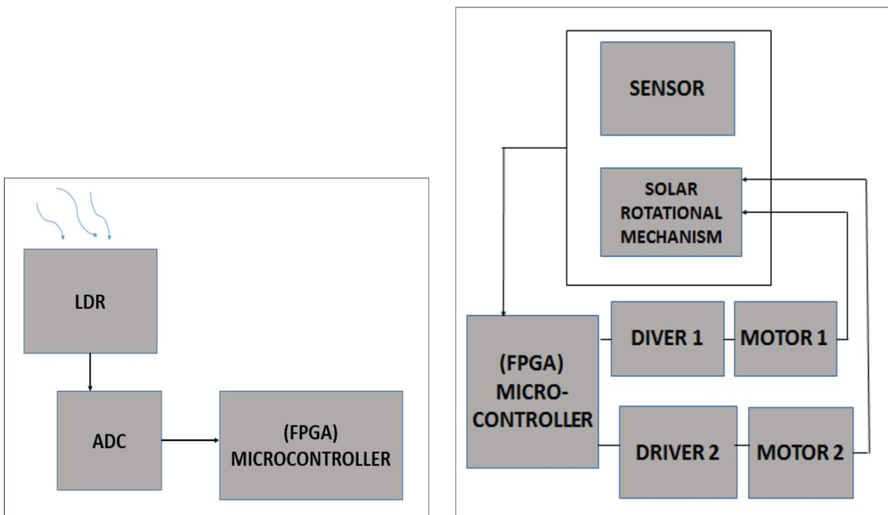
Figure 1. Solar tracking control architecture
