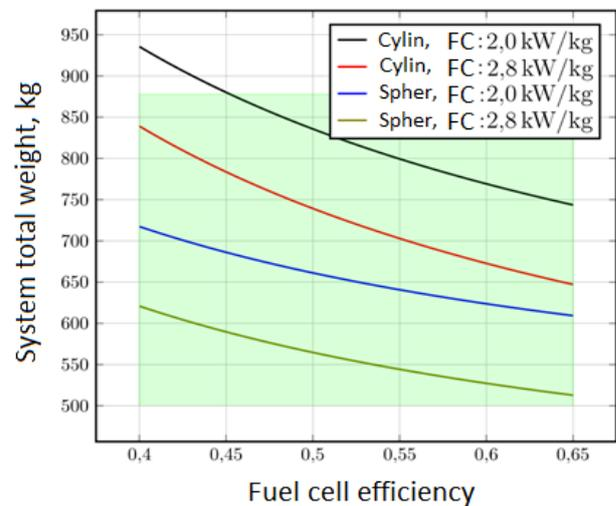
Figure 9. Total weight variation of traction drive
