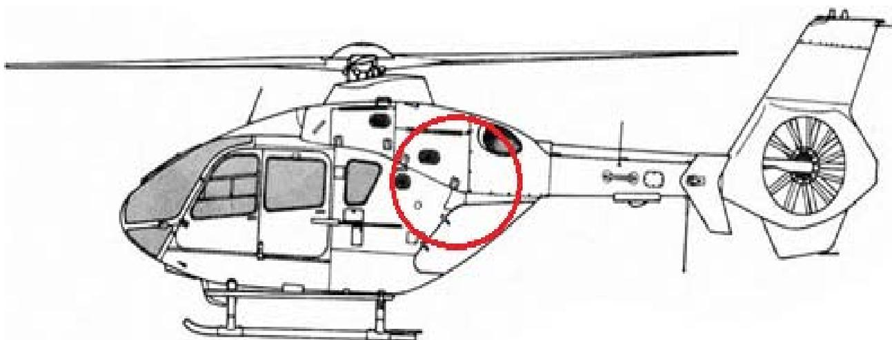
Figure 4. EC135 with interior spherical tank [26]
