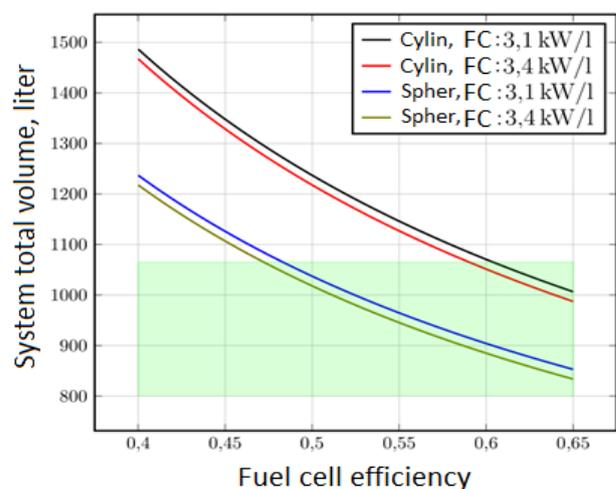
Figure 10. Total volume variation of traction drive
