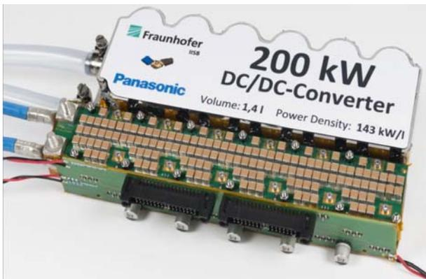
Figure 7. DC/DC-Converter [25]
