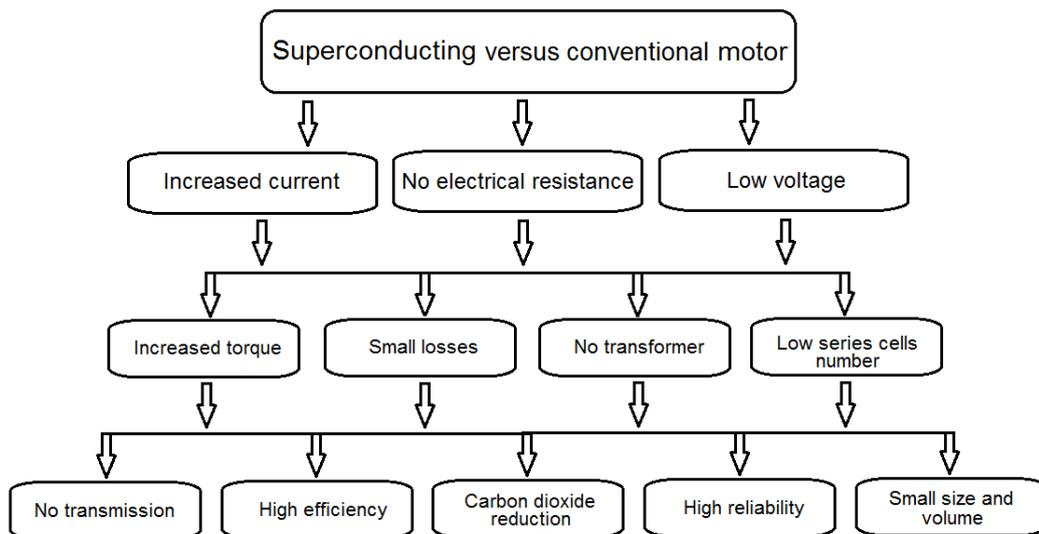
Figure 1.: Advantages of superconducting machines
