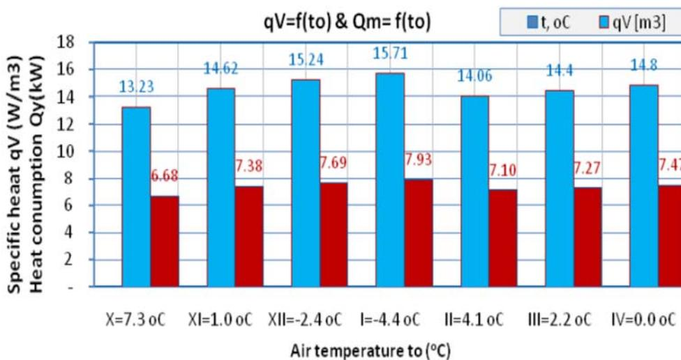
Figure 11. The influence of the air temperature (t<sub>omax</sub> °C, t<sub>omin</sub> °, t<sub>oav</sub> °C) in the specific heat consumption q<sub>v</sub>=f(t<sub>o</sub>) and in the monthly heat consumption Q<sub>yHV</sub>=f(t<sub>o</sub>) from October2015 to April 2016
