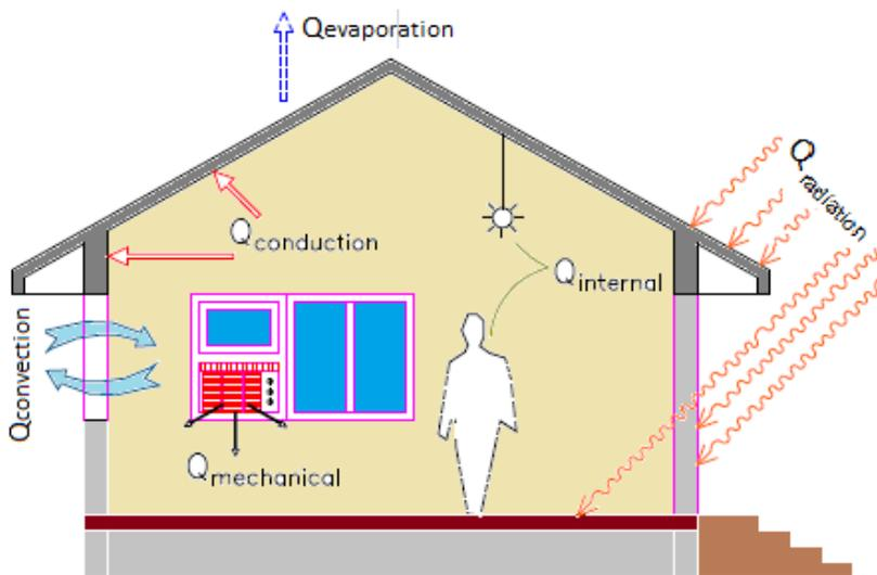
Figure 1. Heat exchange processes
