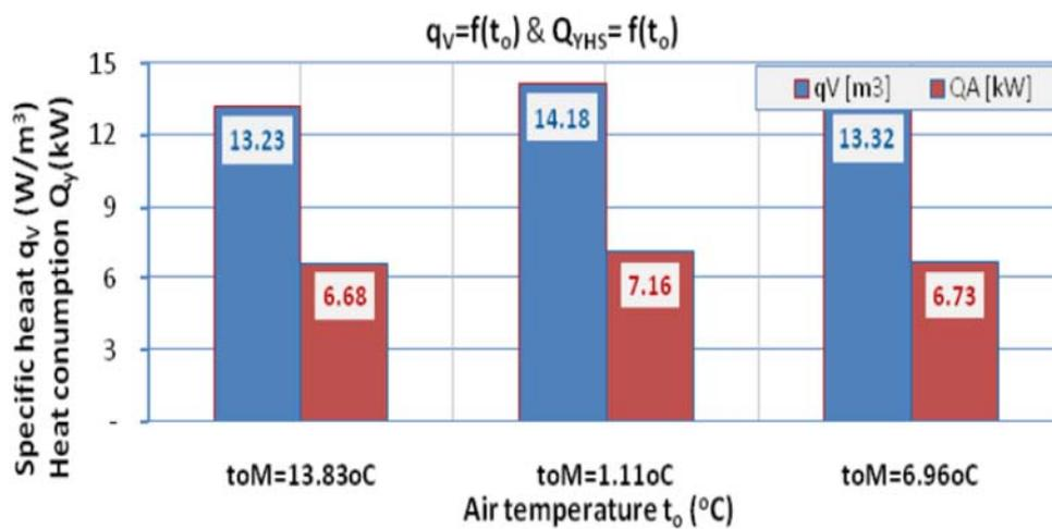
Figure 10. The influence of the air temperature (t<sub>omax</sub> °C, t<sub>omin</sub> °C, t<sub>oav</sub> °C) in the specific heat consumption q<sub>v</sub>=f(t<sub>o</sub>); yearly heat consumption Q<sub>yHV</sub>=f(t<sub>o</sub>) 2015/16
