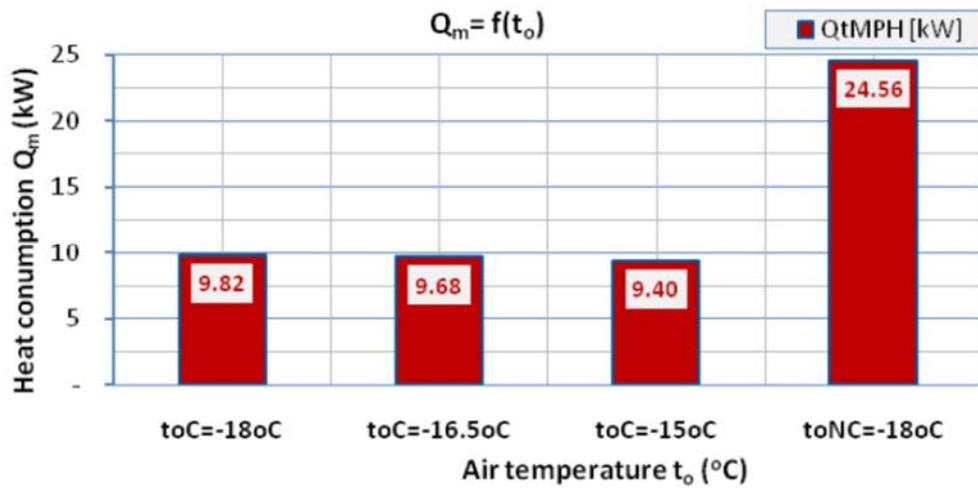
Figure 12. The influence of the air temperature in the heat consumption when the MPH model is designed based on Unified Construction Code ( $t_{oC}$ ) and not based on Unified Construction Code ( $t_{oNC}$ )
