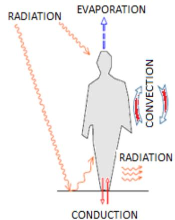
Figure 2. Heat exchange processes a human body
