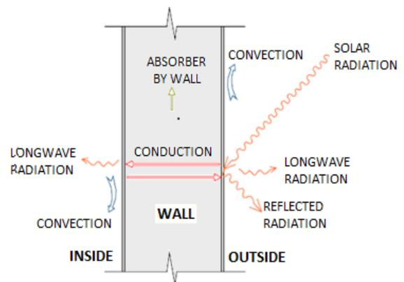
Figure 4. Heat transfer processes occurring in a wall [7]
