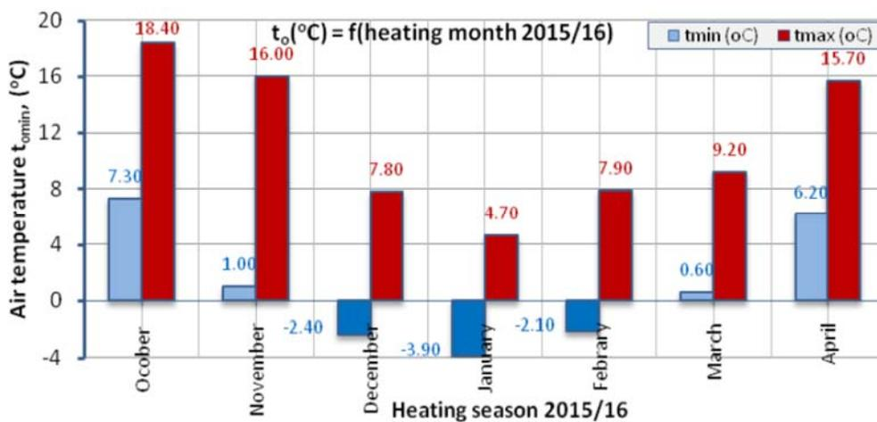
Figure 7. High and low air temperature during heating season in Pristina, 2015/16 [15]
