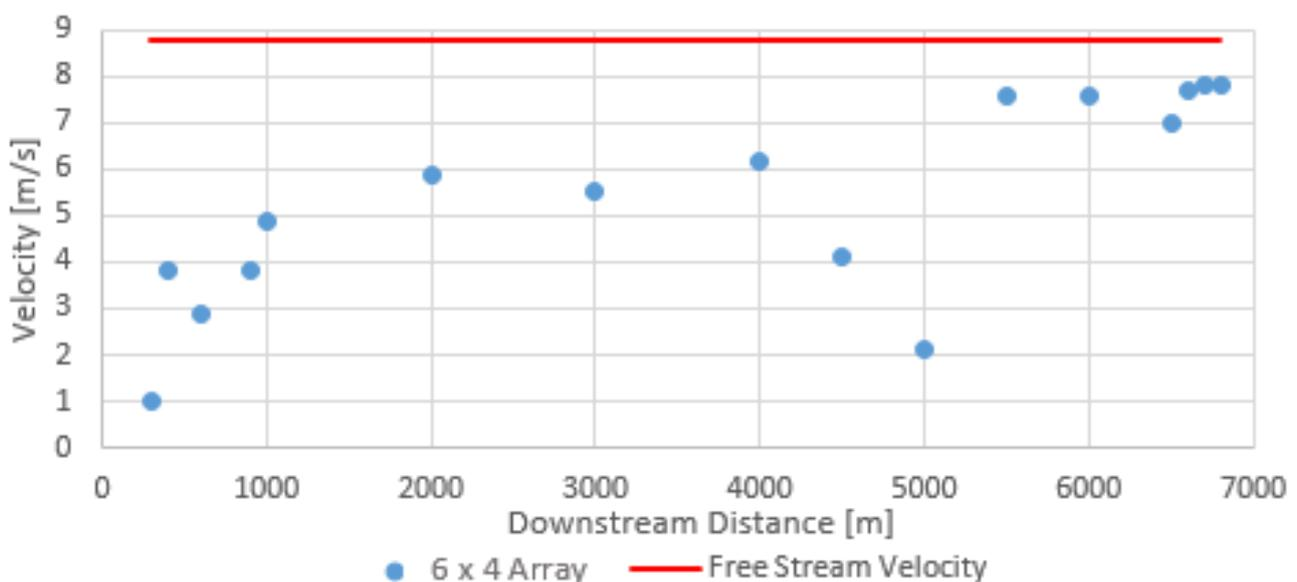
Figure 4. Velocity recovery in a 6 x 4 array wake
