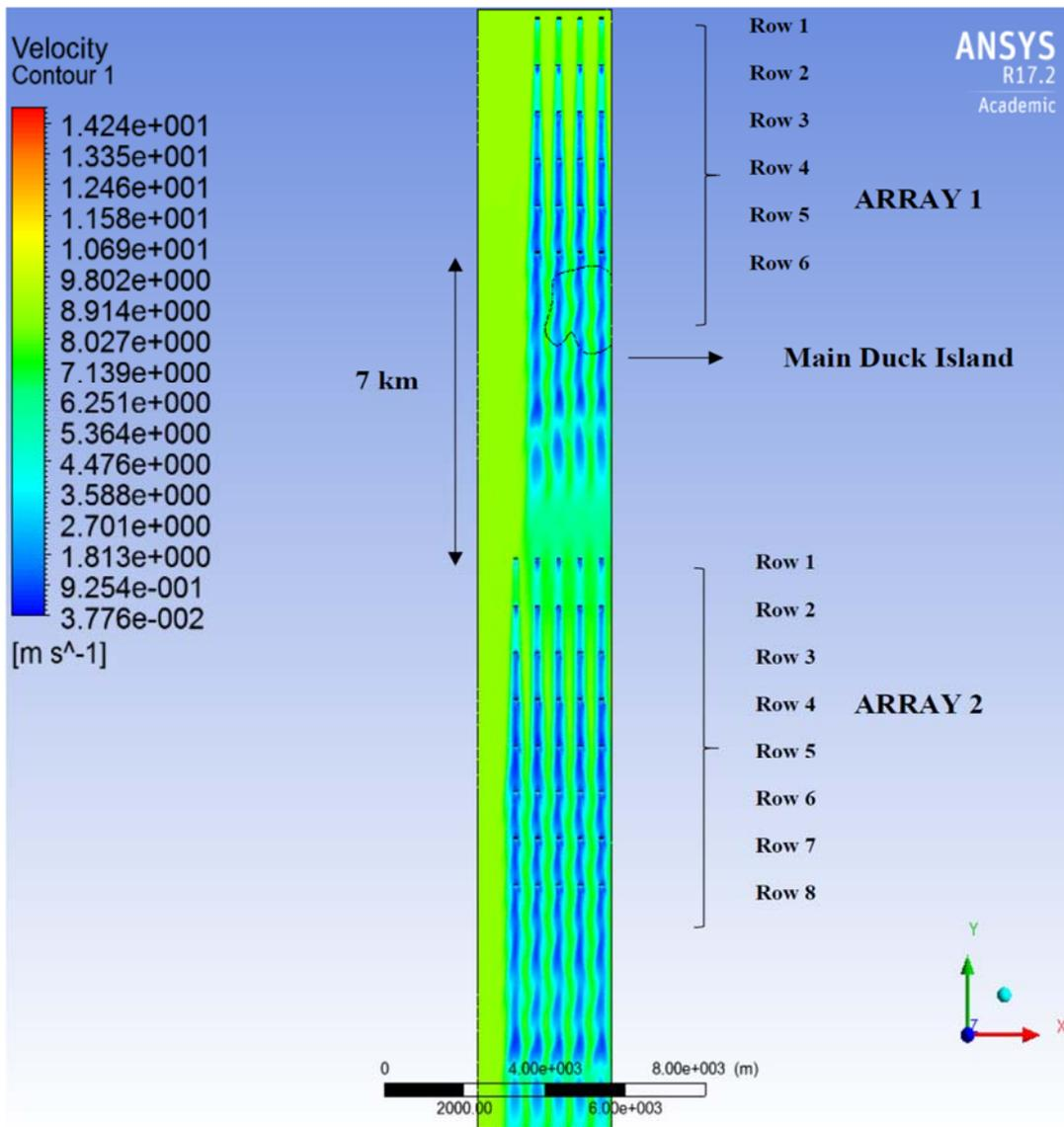
Figure 5. Velocity contour plot of the two-array simulation
