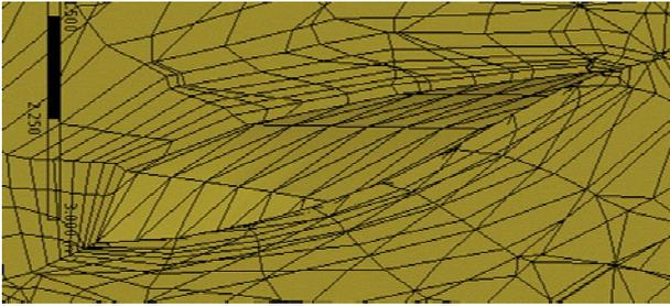
Figure 2. Hybridized mesh surrounding a blade element
