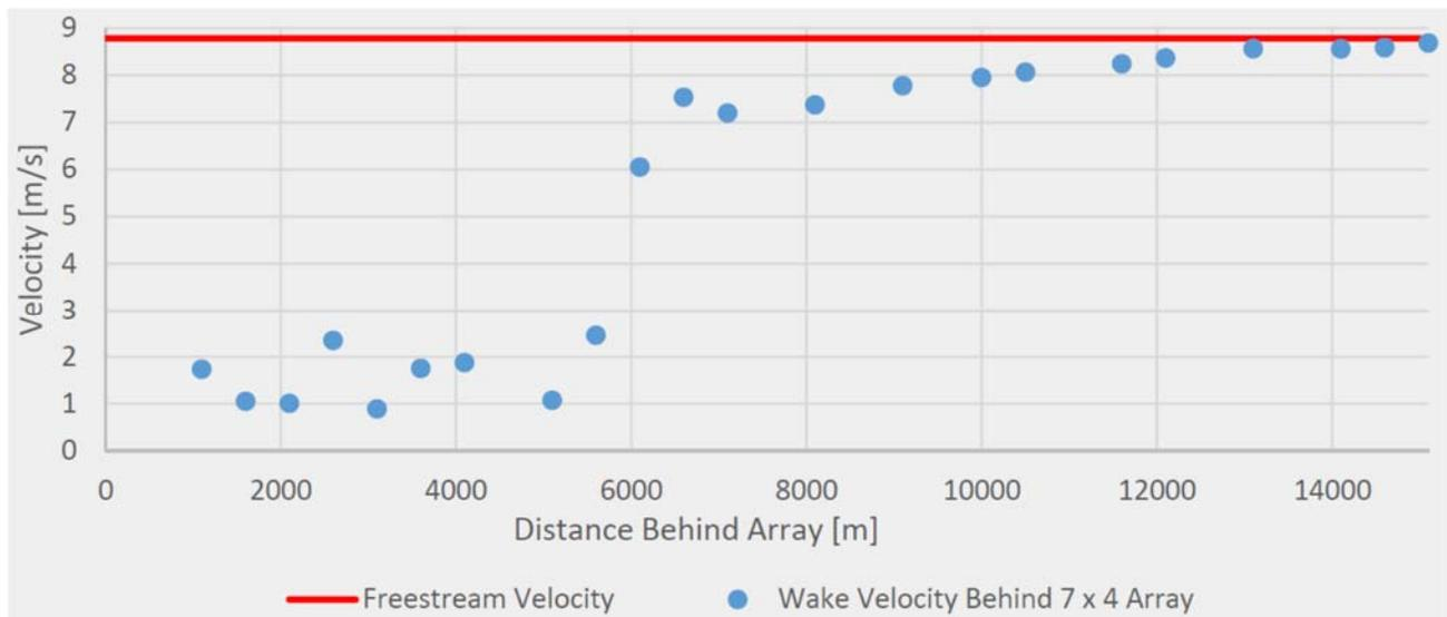
Figure 7. Velocity recovery in a 7 x 4 array wake
