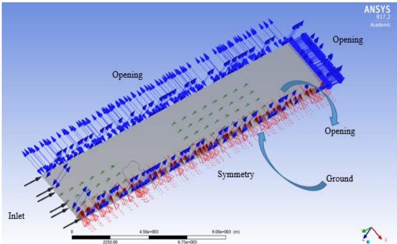
Figure 3. Boundary conditions of the two-array simulation
