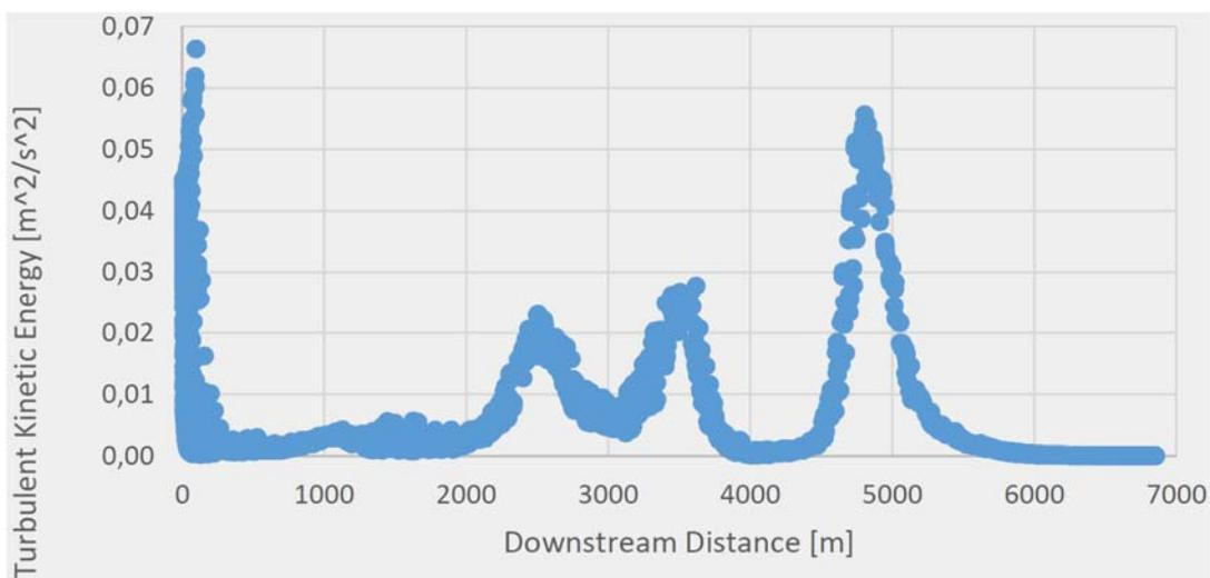
Figure 6. Turbulent kinetic energy in the wake of a single turbine in array 1
