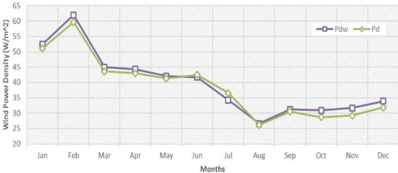
Figure 3. Variation of monthly wind power computed at 10 m height by using two different methods
