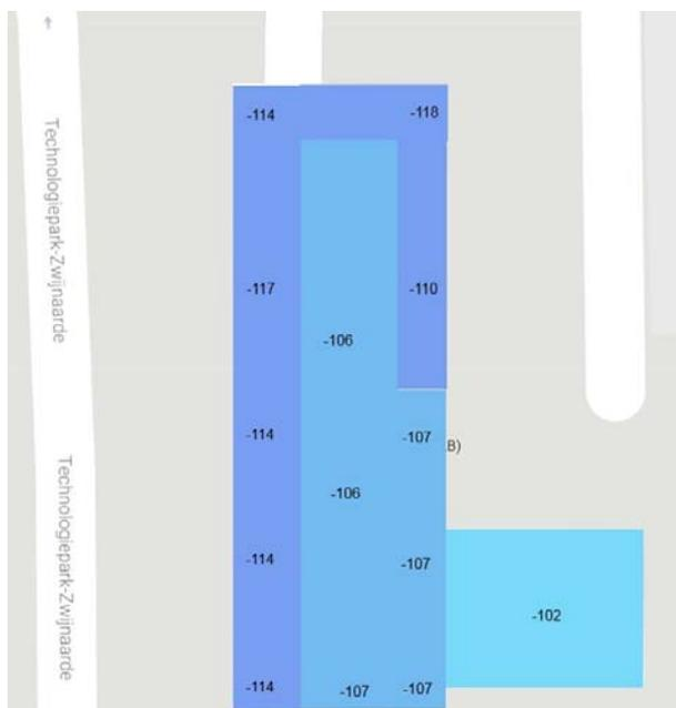
Figure 3. LoRaWAN coverage of the basement floor of a campus building
